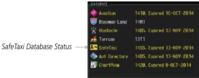
Figure 5-20 Power-up Page, SafeTaxi Database
