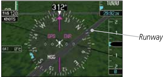
Figure 5-37 Depiction of Runway with a Loaded Flight plan
