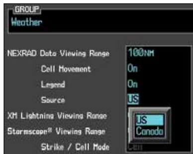
Figure 3-27 NEXRAD Weather Source Selection
