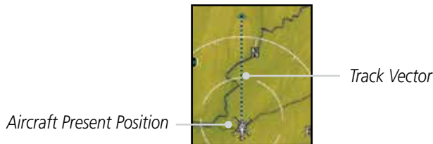
Figure 3-14 Navigation Map Track Vector
