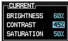
Figure 3-67 External Video Contrast Adjustment
