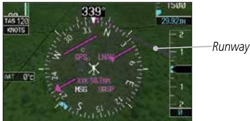
Figure 5-38 Depiction of Runway Not in Loaded Flight plan
