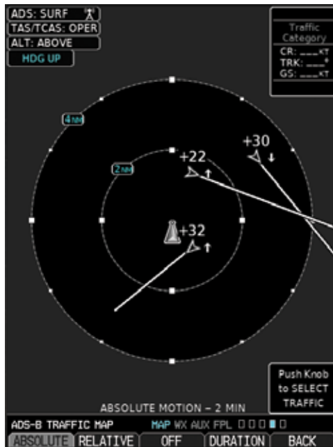
Figure 4-30 Absolute Motion (White Vectors)
