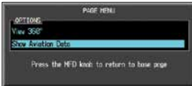
Figure 4-7 Show/Hide Aviation Data on the Terrain Page
