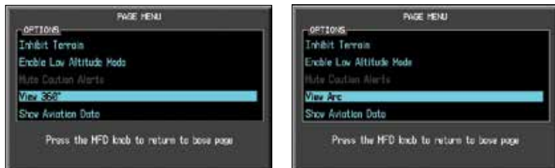
Figure 4-14 Terrain-HSVT Page Menu Viewing Selections
