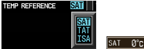
Figure 3-43 Outside Air Temperature Selection
