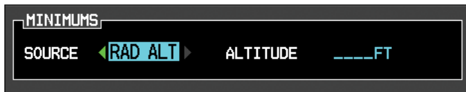
Figure 5-14 Minimums Source Selection
