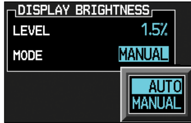
Figure 3-39 Aux Mode Display Brightness Mode Selection
