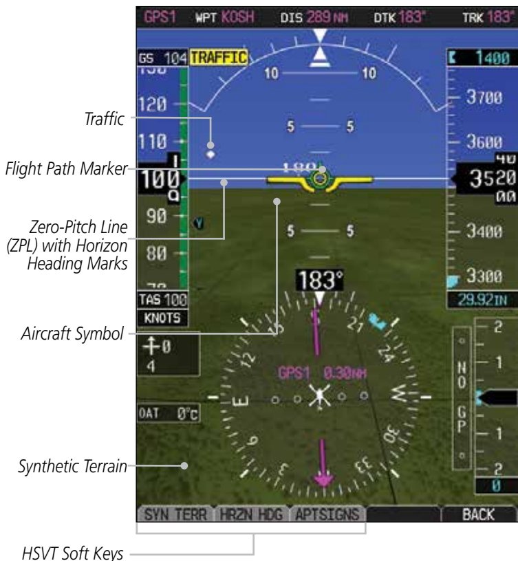
Figure 5-34 HSVT on Primary Flight Display
