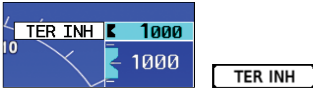
Figure 4-17 Terrain-HSVT Alerting Disabled (Alerts Inhibited) Annunciation (PFD & MFD)
