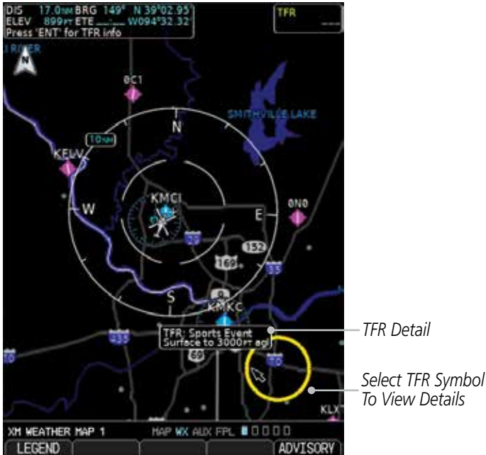
Figure 4-56 XM Weather - TFRs
