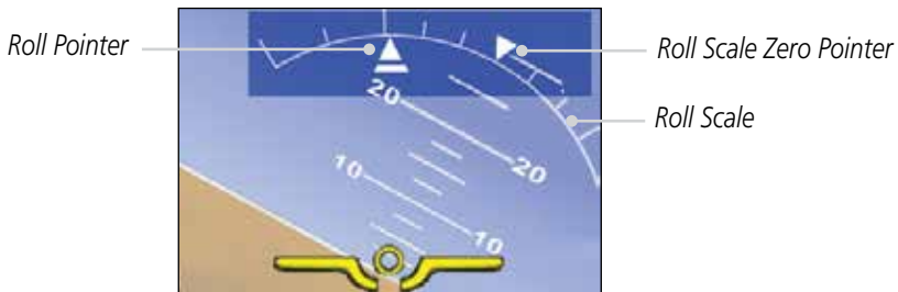
Figure 2-11 Attitude Indicator with a Ground Pointer Configuration in a Left Turn
