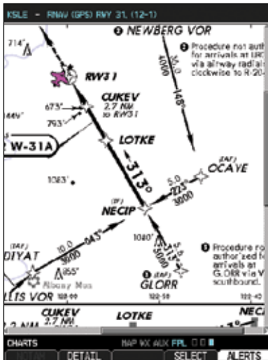
Figure 5-11 Zooming and Panning Around a Chart
