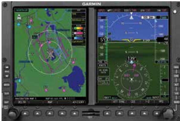
Figure 1-2 GDU 620 PFD and MFD
