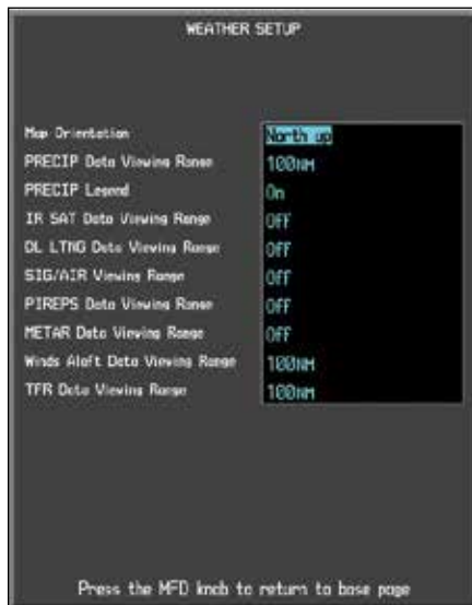
Figure 4-67 Weather Data Link Setup Menu Options
