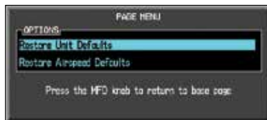
Figure 3-37 Aux Mode System Setup Page Menu
