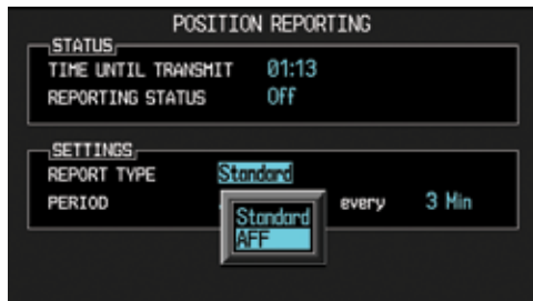
Figure 3-75 Select Automatic Flight Following (AFF) Reporting Type
