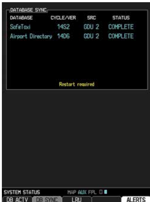
Figure 3-57 Database Transfer Complete
