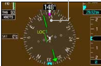
Figure 2-32 Auto-Slewing HSI with Localizer Backcourse Loaded (Shown with Corresponding Approach Plate)
