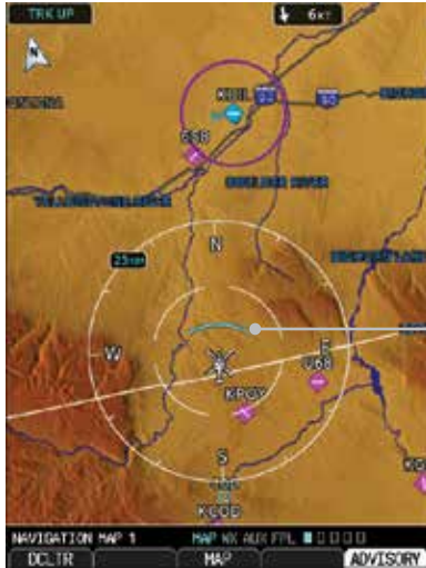
Figure 3-23 Selected Altitude Range Arc
