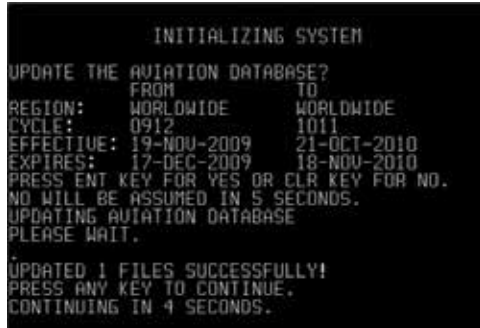
Figure A-2 Database Loading Completed
