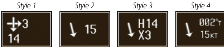
Figure 2-37 Wind Vector Style
