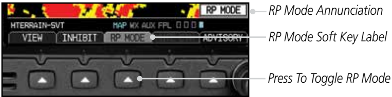
Figure 4-21 Enable or Disable RP Mode on the Terrain-HSVT Page
