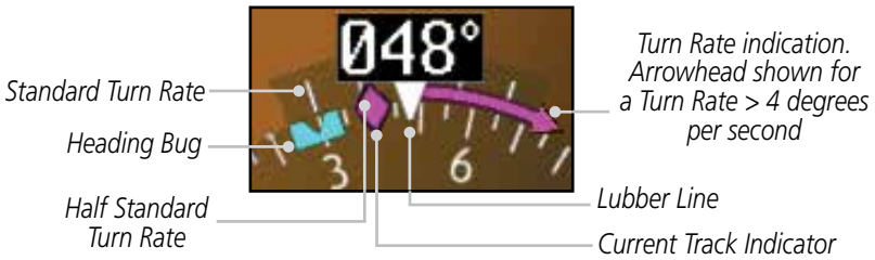
Figure 2-25 Turn Rate Indicator and Trend Vector
