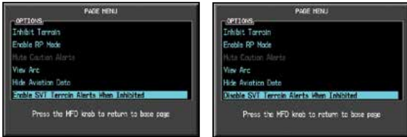
Figure 4-24 Enable/Disable SVT Terrain Alerts When Inhibited
