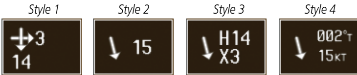
Figure 3-41 Wind Vector Style
