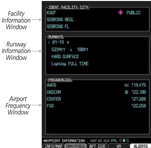
Figure 3-101 Flight Plan Waypoint Info Detail
