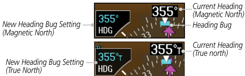
Figure 2-24 Heading Bug Setting
