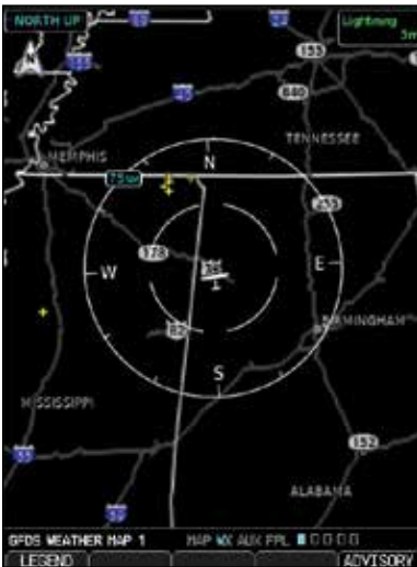
Figure 4-79 GFDS Data Link Lightning and Legend
