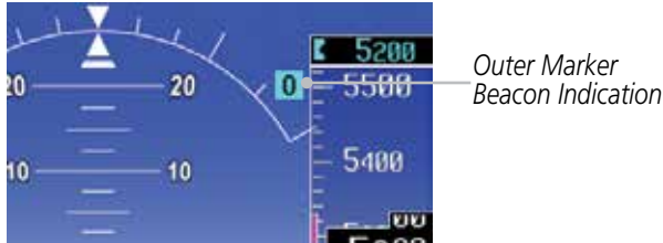
Figure 2-39 Marker Beacon Location
