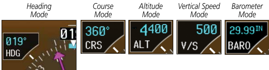
Figure 1-17 Selection Modes Adjusted with the PFD Knob
