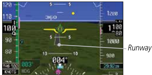
Figure 5-39 Depiction of Runway with Loaded Approach
