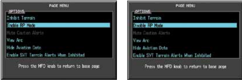
Figure 4-20 Enable or Disable RP Mode on the Terrain-HSVT Page
