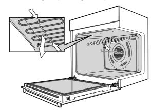
Rotating latch models - rotate latch 180 degrees and the grill element will drop down freely. After cleaning, raise the grill element and secure by rotating the latch back 180 degrees.
