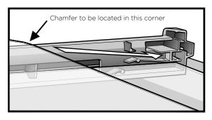
Insert the black bordered glass panel into the upper position, ensuring the painted surface is facing the downside as per the image below.
