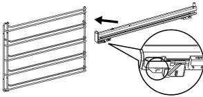
The shaded wires indicate the wire the slide can be mounted on. Fit slide rear clips to the rear of wire at an angle as shown below.
