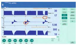
Freeze Waveform & Measure Peak Expiratory Flow
