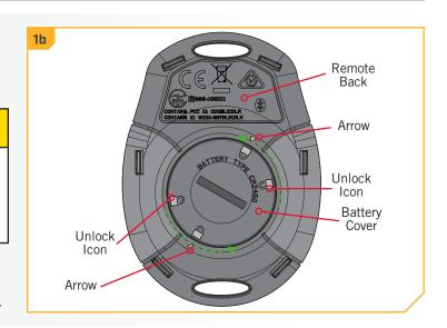
Remove the Battery Cover and old battery and replace with a new CR2450 coin cell battery. Note the proper polarity of the battery.
