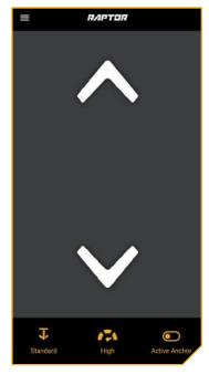
The Raptor Control Screen when one Raptor is paired to the device. This screen differs slightly when two devices are paired.
