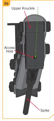
With the Spike removed, take the new Spike and place it back into the Upper Knuckle. Note that the top of the Spike has two a Half-moon Grooves perpendicular to the length of the Spike. This helps orientate the Spike into the Upper Knuckle in the correct direction to be captured by the Hex Bolts. Replace the Spike and align the holes in the top of the Spike with the Half-moon Grooves on the top of the Spike. The logo on the Spike molding should be facing away from the Raptor.
