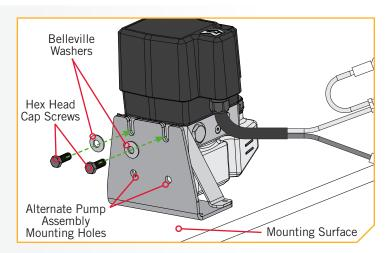
**NOTICE:** The U-shaped slots and the larger holes on the Pump Bracket may be used to mount the Pump Assembly to the bracket. The holes used will depend on individual mounting circumstances.
