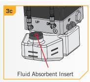
**NOTICE:** Raptor is 100% quality and performance tested with hydraulic fluid. Discard residual fluid absorbent insert. For shipping purposes only.
