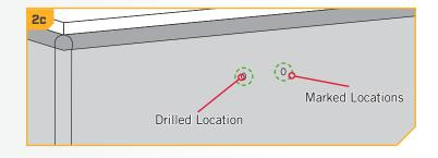
**NOTICE:** When drilling holes into fiberglass, it is helpful to first cover the surface with masking tape. Use a 5/16" Drill Bit when drilling into Fiberglass for the Pilot Holes. Masking Tape will help keep the boat surface unmarked and help with cleanup. Cover the surface and then mark the location to drill. Once the pilot holes are drilled, remove the masking tape before continuing installation.
