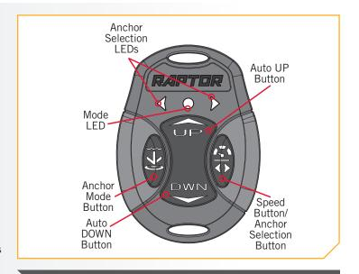
**NOTICE:** When two Raptors are paired, the anchor of the selected Raptor will deploy. The selection can be Port, Starboard, or both.
