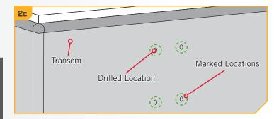
**NOTICE:** When drilling the marked holes, make sure that the drill bit is perpendicular to the Transom/Stern of the boat and that the holes are being drilled straight. Not drilling the holes straight will give the mounting hardware a poor fit.
