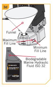
**NOTICE:** Minn Kota recommends using Biodegradable Marine Hydraulic Fluid ISO 32 (Part #2357700.) If additional Hydraulic Fluid is needed, order online at minnkotamotors.com or find an equivalent ISO 32 biodegradable marine grade hydraulic fluid.
