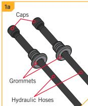
**NOTICE:** If routing the Hydraulic Hose through an established routing system on the boat, the Grommets may be removed.
