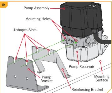
**NOTICE:** The Pump Assembly must be mounted vertically. If adjustments to the mounting need to be made, rotate the position of the Two-piece bracket to accommodate the necessity to keep the pump vertical.
