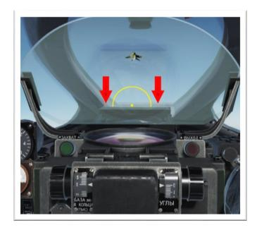
Standard solutions are to maintain the sight Caged until the Distance Measurement, then Uncage and Fire over the established aiming point, or use a Caged Sight and aim by the Pilot's own predictions.
