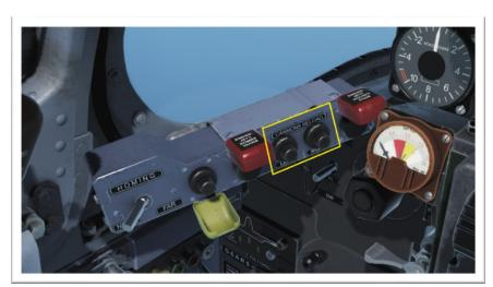
3. After every press, check that the corresponding Red Lamp, indicating an armed cannon, is illuminated on the lower Main Instrument Panel above the Ammunition Counters.
