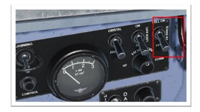
3. After the warm up time has expired, put the switch in the On position.
