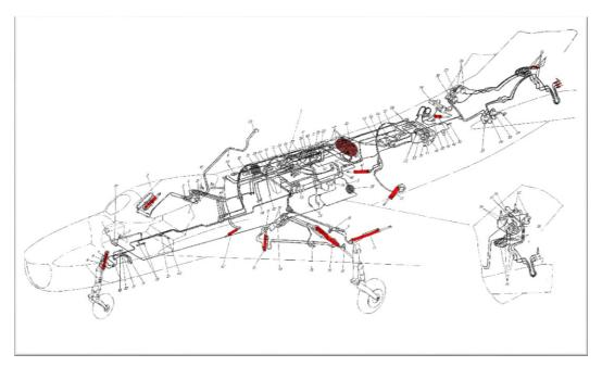
Both systems are independent and operate all the Hydraulic consumers by separate chambers and Check Valves. So, in case any of them fails, the other will take over the functions.
