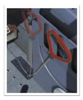
LANDING GEAR EMERGENCY DEPLOYMENT HANDLE
