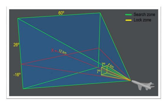
The RP-5 is heavily affected by Ground returns at Low Altitude, making it impossible to use at Altitudes below 2,000 meters. The Radar has an Altitude Mode Switch, on the Main Instrument Panel, which disconnects the Search Antenna and reduces the Track Antenna Range from 4,000 to 1,200 meters. This allows for Automatic Aiming Solutions from 2,000 meters down to 1,000 meters in Daylight Conditions. This transforms the RP-5 into a Radio-Rangefinder.
