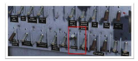
2. On the RP-5 control panel, located on the left panel, put the radar mode control switch in the Standby Position.
