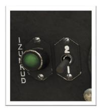
RP-5 RADAR EMITTING LAMP & ALTITUDE MODE SWITCH
