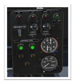
3. Turn On the "Arm Bombs Fuse" Switch. The Red "Exp" (explosion) Lamp should illuminate.
