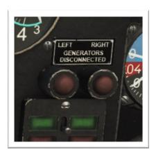
LH/RH DC GENERATOR FAILURE LAMPS
