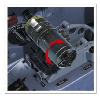
5. The Distance introduced manually can be checked on the Target Distance Indicator to the left of the ASP-5N Sight.
