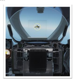
During this process, as the Gunsight Gyros are Uncaged, it may be possible that during high G maneuvers, the reticle moves too far down, disappearing from the Sight Field of View. While this may not be an issue at Short Range, because Bullet deflection is not relevant, it may prevent effective engagement of Targets at Medium to Far Distances as in this case it will be impossible to introduce the correct Distance for a good Aiming Solution.
