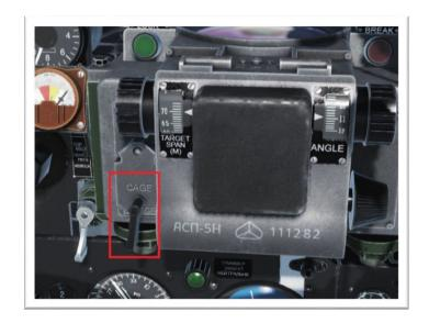
4. Having selected the Target Wing Span, change the Aiming Reticle Distance by rotating the Throttle Handle backwards and forwards, check the change in the Diameter of the Outer Circle.
