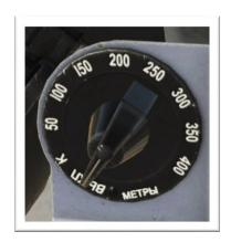
RV-5 RADAR ALTIMETER MINIMUM ALTITUDE SELECTOR
