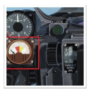
6. When pursuing the target, rotate the Throttle Handle, so the wingtips of the Phantom touch the borders of the Outer Circle. This ensures the correct distance to target is introduced into the Sight. As the Distance to Target changes, this value can be adjusted, the Sight will calculate the Angular Velocity value and project an Aiming Solution. Open fire while maintaining the Center Dot over the Target.
