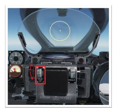
3. Uncage the Sight Gyro by turning the Cage/Uncage Lever. This allows the Aiming Reticle to move freely allowing Gunsight Gyro Precession.
