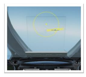
6. As the Distance to Target approaches 300 meters, the Red Break lamp will illuminate, instructing the Pilot to Turn away and leave the attack run to avoid a collision. After 3 seconds the Lock will be dropped, as well as all Aiming Solution.
