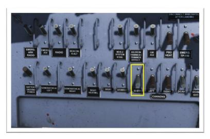
2. On the ASP-5N Control Panel, put the Armament Mode Selector in Rocket Pods (P.C).
