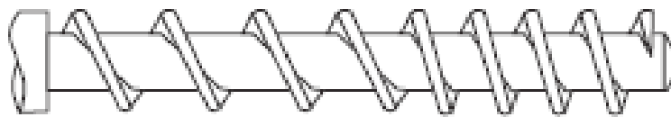
Figure 19. Zero Compression Screw (Variable Pitch)
