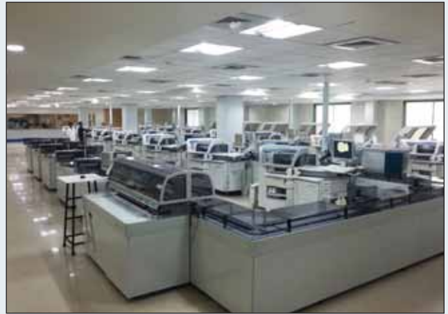
The world's longest automation track installed by Siemens at Thyrocare Technologies is boosting the availability of in-vitro diagnostic testing services.
