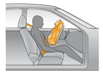
In a moderate-to-severe frontal crash, the seat belts lock to restrain the occupants, and tensioners tighten the front seat belts. Front airbags help slow occupants' forward movement and have been proven very helpful in reducing serious head and chest injuries. Front airbags inflate and deflate in a fraction of a second, so fast that many people do not realize their airbag deployed until they see it in front of them.
