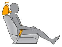
Adjusting a head restraint so the center is level with the back of the occupant's head (or as high as possible for taller people) can help reduce injuries during a rear impact. In vehicles equipped with active head restraints, the restraint will move up and forward a little when enough pressure is applied against the seatback.
