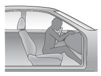
In a 30 mph, head-on crash into a barrier, a vehicle decelerates to a stop in about 1/10th of a second, less than the blink of an eye. What happens to an occupant during this time? Without a seat belt or an airbag, the occupant will continue forward at 30 mph until they strike the interior of the car with enough force to cause serious injuries.
