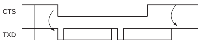
Figure 36-28. Transmitter Behavior when Operating with Hardware Handshaking
