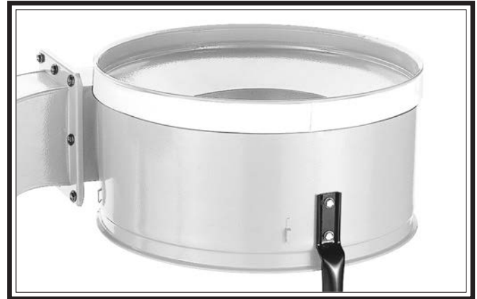
Figure 74. Tape applied to top rim of collector.
