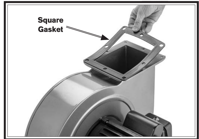
Figure 12. Square gasket in place on impeller rim.
