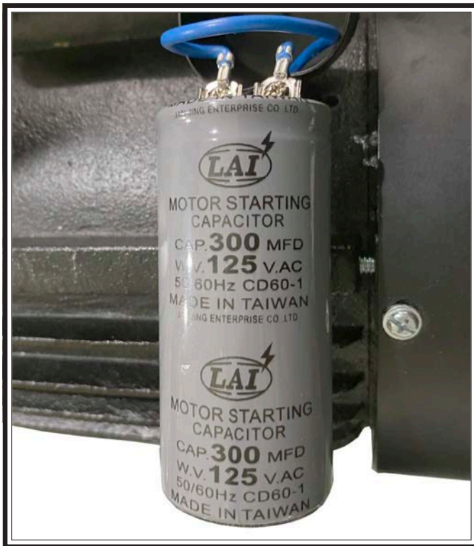
Figure 85. SB1100 start capacitor.
