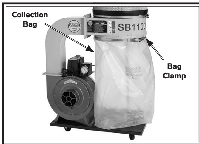
Figure 26. Collection bag installed to dust collector.
