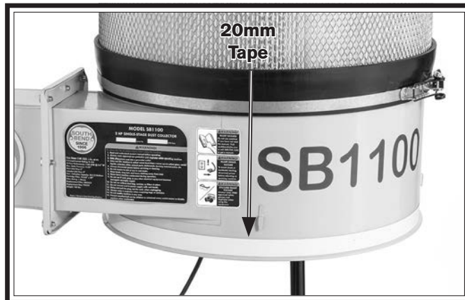
Figure 25. Tape applied to bottom rim of collector.
