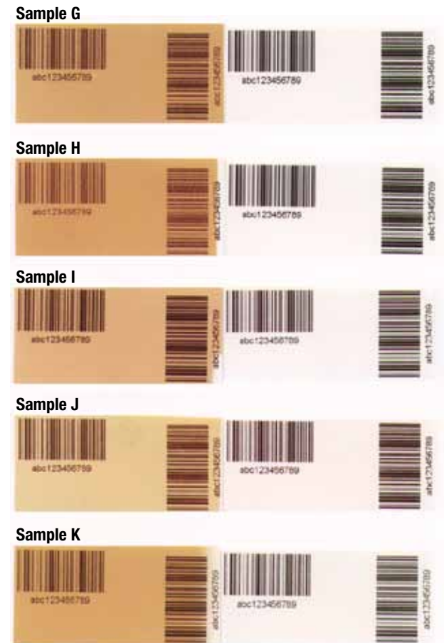
Figure 5. UV light exposure seven-day test results
