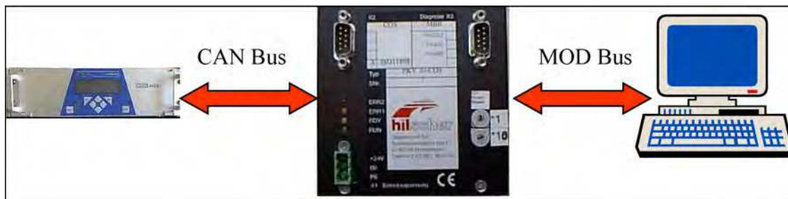
Fig. 172 Connection the SUPREMA to external systems using a Modbus RTU gateway
