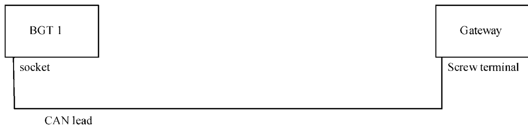
Fig. 176 Connection Suprema Gateway CAN/Profibus DP
