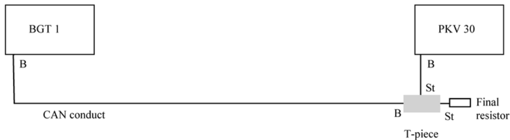
Fig. 173 Connection Suprema Gateway CAN/Modbus RTU
