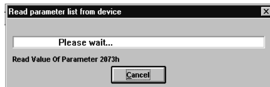
Figure 18: CMD tool reads in device parameters, i.e. PCP communication is ok
