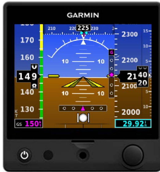
Figure 1-1, G5 Electronic Flight Instrument (Attitude)
