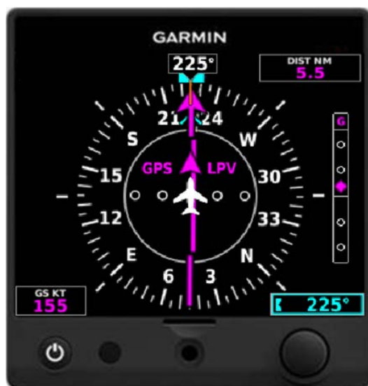
Figure 1-3 G5 Electronic Flight Instrument (DG/HSI)
