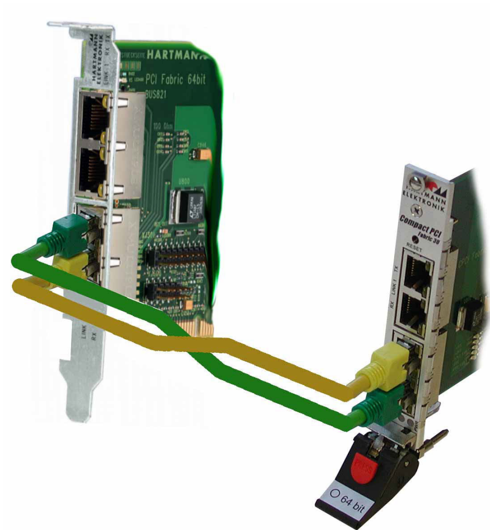
Figure 7-25: Cabling of the R&S TS-PSC0 components.
