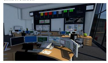
All incoming emergency calls go through the control station where they are received and processed by a dispatcher. From here, the emergency services needed for each call are alerted and dispatched to the scene automatically. During the operation, the control station will receive updates on the operation itself and the vehicles. This is done via the status transmitter and the digital radio communication system.
