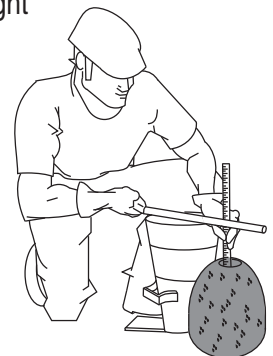
Figure 68-F. Slump Test (Measurement)
