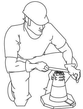
Figure 68-D. Slump Test (Removing Excess Concrete)
