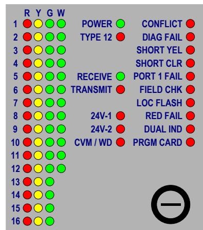
The indicator for a field input will be on if the RMS voltage over the last 33 milliseconds (two cycles of AC power) is above the threshold for that type of input. (See Section [3.2](#) for the voltage levels for each type of input.)
