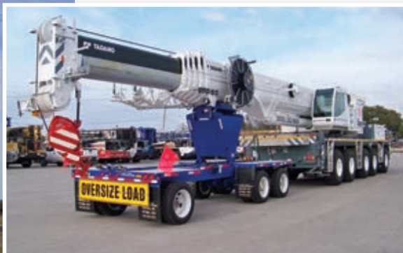
Sims Crane transports its Tadano ATF180G-5 using a three-axle Nelson boom dolly.
