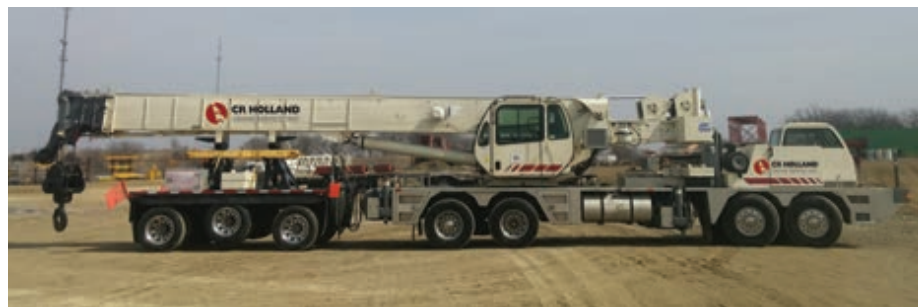
The first boom dolly produced by HMR Supplies was for its sister crane company CR Holland in the mid-2000s. Since that time, HMR created a product line that includes two-axle, three-axle, and four-axle boom dollies.
