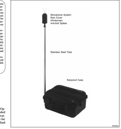
Portable Noise Monitoring Option Type 3571 allows all-weather monitoring using a Type 2236 Precision Integrating Sound Level Meter. The system can operate unattended for more than three whole days. Batteries can be changed without interrupting measurements, thus allowing long-term monitoring.
