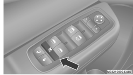
Window Lockout Switch
