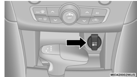
Front Power Outlet
