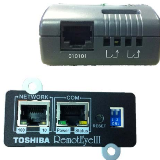
Figure 36: EMD RemotEye III Installation
