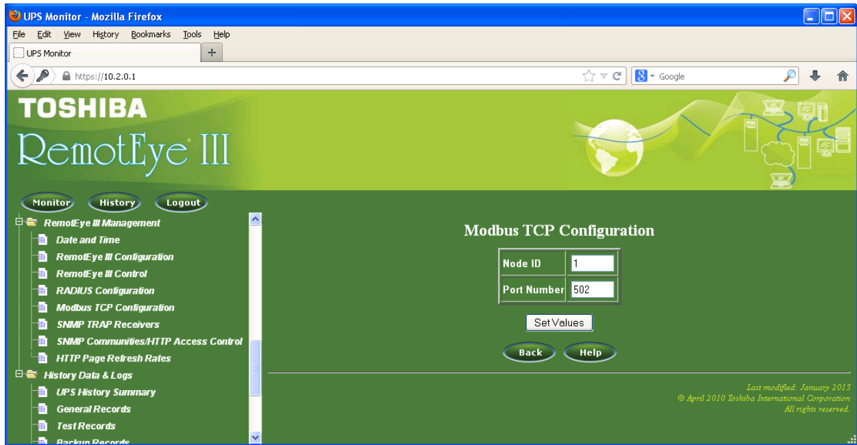
Figure 51: RemotEye III Modbus TCP Configuration
