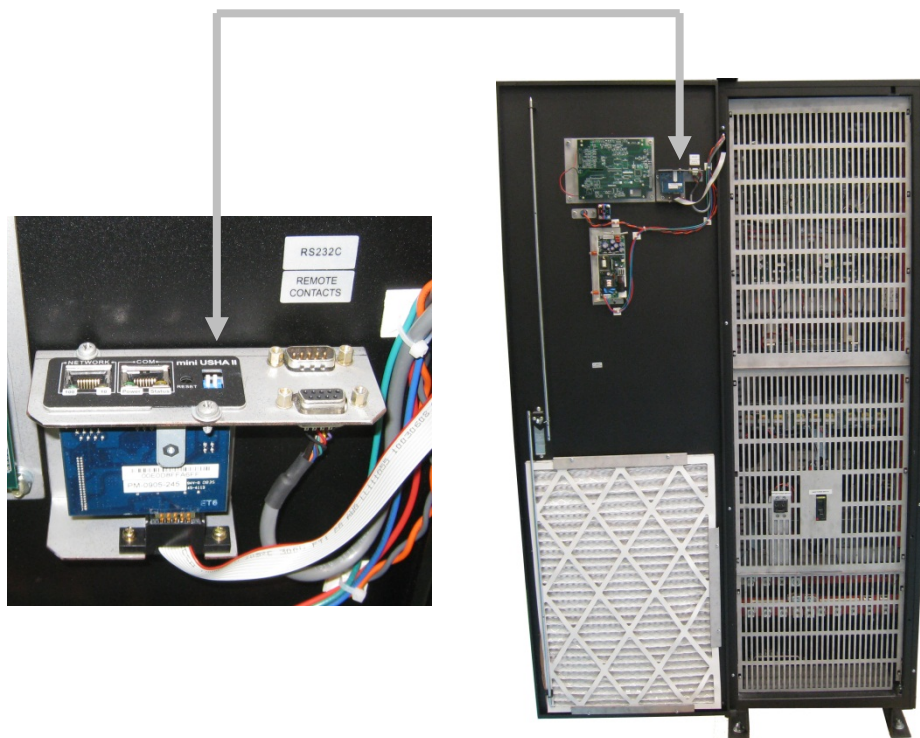
Figure 12: RemotEye III in 4300 UPS
