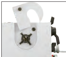
4 Brass-Tipped Spider Bolts for Supporting Barrels
