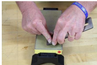
Plane Iron – sharpening – across the stone's surface
