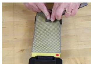
Plane Iron – sharpening – across the stone's surface
