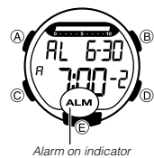
Alarm on indicator
