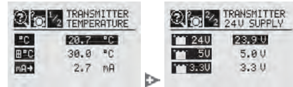
Figure 171. Transmitter Temperature and Supply Voltage Screens
