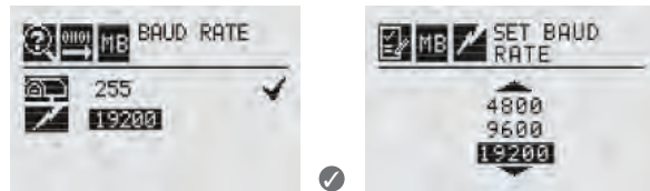
Figure 141. Set Baud Rate Screens
