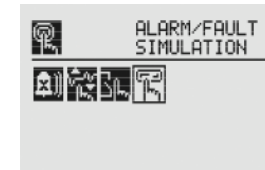
Figure 156. Alarm/Fault Simulation Screen
