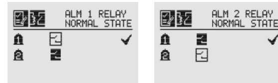
Figure 186. Relay State Screens
