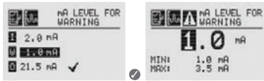
Figure 103. Set mA Levels for Warning
