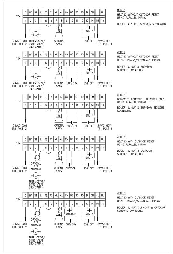
Figure 3 – Field wiring to terminal block TB4
