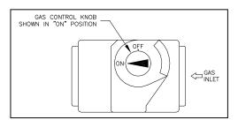
NOTE: On some gas valves the knob cannot be turned to "OFF" or "ON" position unless knob is pushed in slightly. Do not force.
