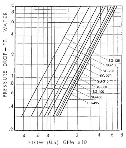
SG Heat Exchanger Pressure Drop Graph
