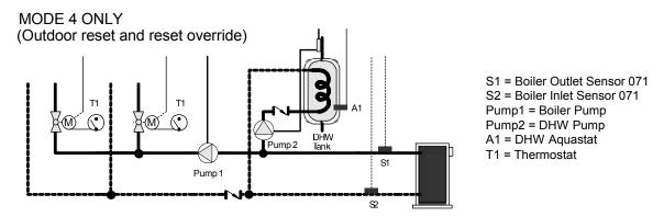
Figure 4 – Typical piping diagram in Mode 4
