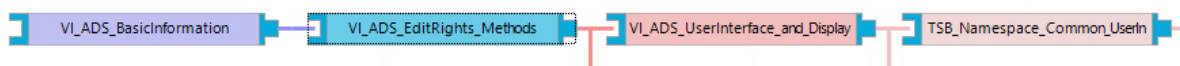
Figure 24: Diagram of Permissions Group Hierarchy (Direction of Inheritance from Right to Left)
