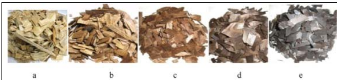
Figure 2.17: Effect of temperature on the color of torrefied pine chips at (a) Raw, (b) 225 °C, (c) 250 °C, (d) 275 °C, and (e) 300 °C
