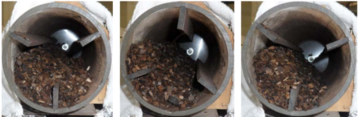
Figure 5.3: Reactor surface covered by solid at overloading case at different time
