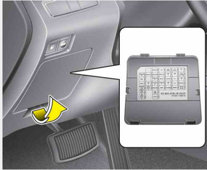
Inner panel fuse panel
