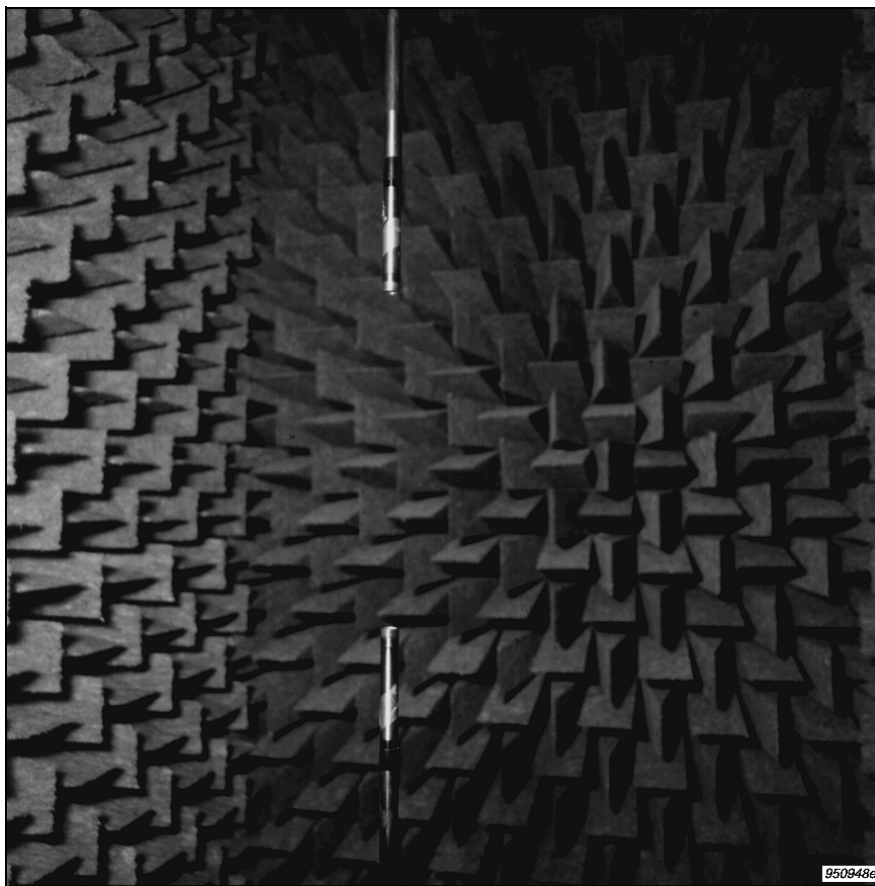
Fig.1.4 Anechoic chamber used for measurement of free-field response
