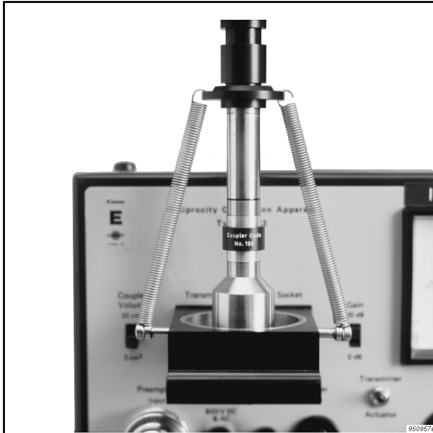
Fig.6.3 Reciprocity calibration. Microphones are held “face to face” by a spring-loaded yoke
