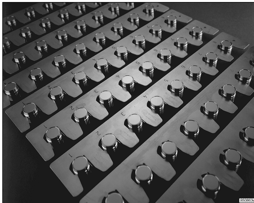
Fig. 1.7 Pre-polarized microphones nearing the end of production
