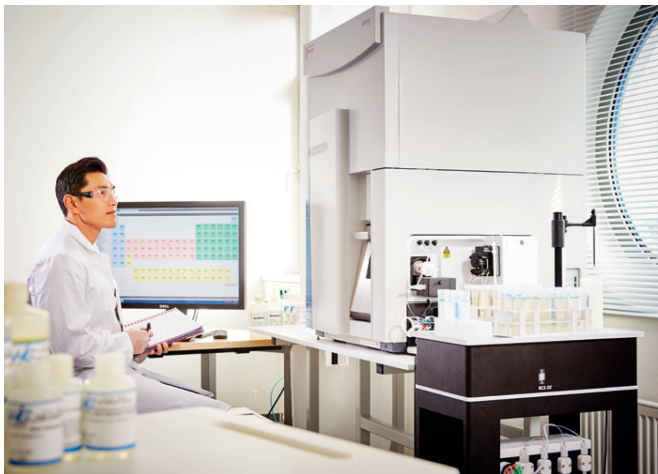
Figure 9. ESI prepFAST Auto-dilution system integrated to iCAP RQ ICP-MS
