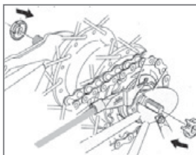
Fig. 70. Installation of adjusting washers
