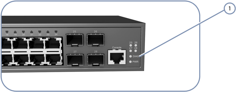
1 System Status LEDs.
