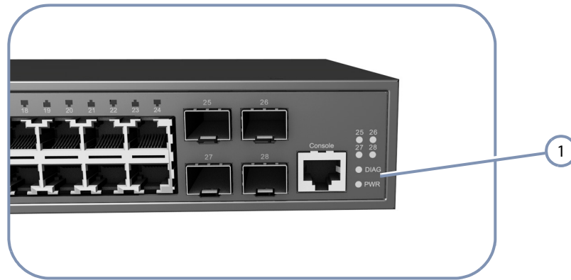
1 System Status LEDs
