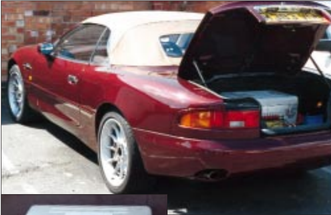
Above: The CR7 displays and stores vehicle test data from a prototype Aston Martin DB7. Left: Closeup of ENC 7F modified with custom connectors. Photos courtesy of Aston Martin, Ltd.
