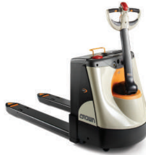
WP 3000 Series Walkie Pallet Truck Load Capacity: 1600 & 2000 kg Lift Height: Up to 750mm
