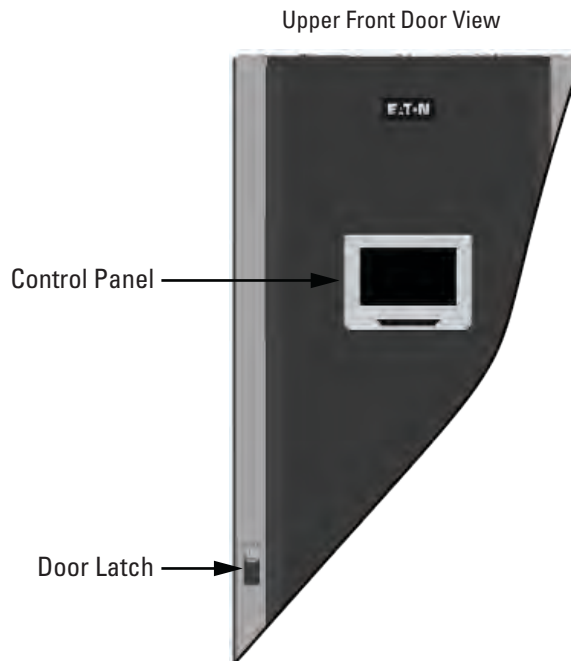
Figure 51. UPS Control Panel Location
