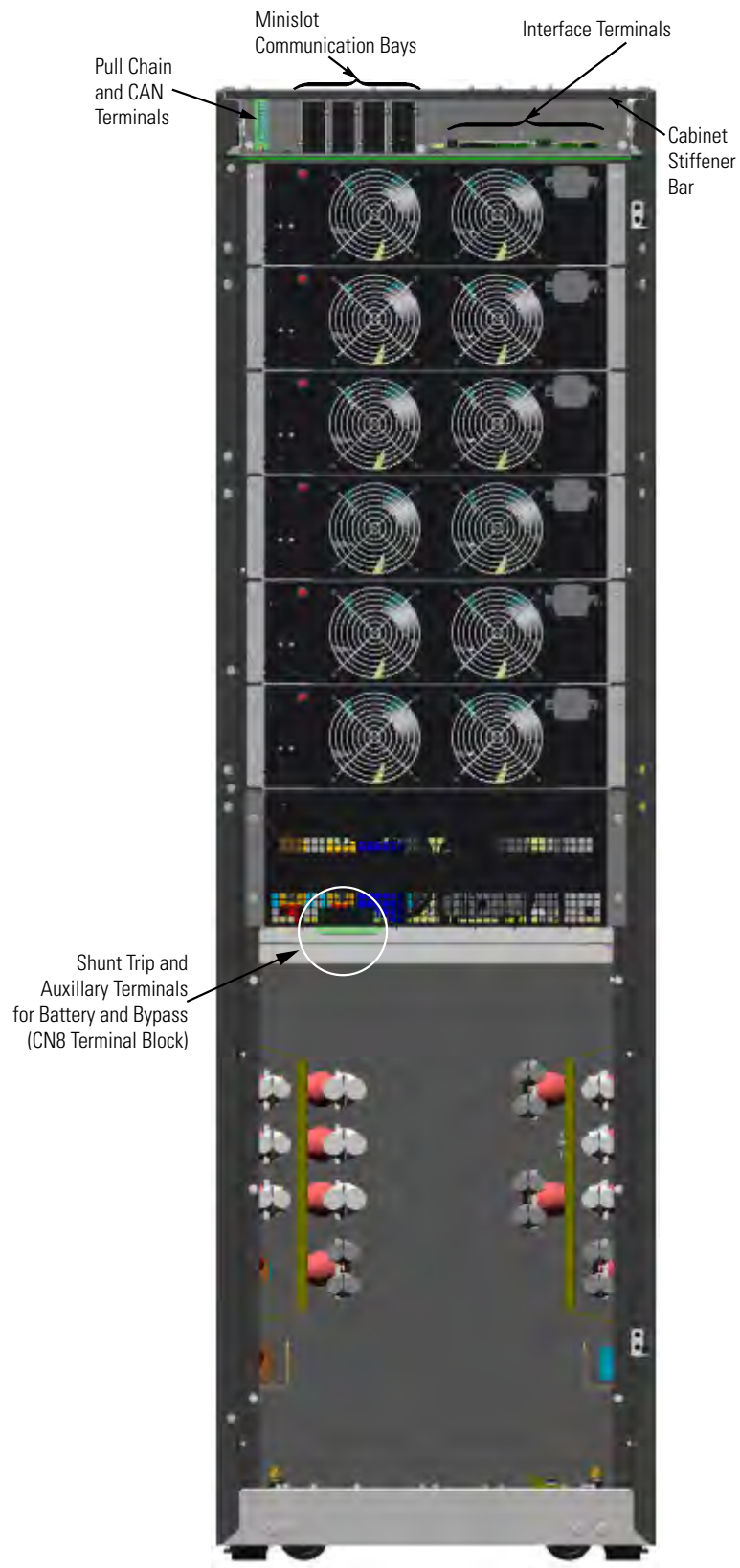
Figure 29. Interface Terminal Locations
