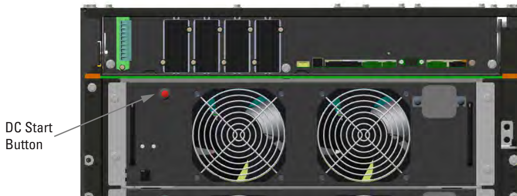
Upper Cabinet View of UPS
