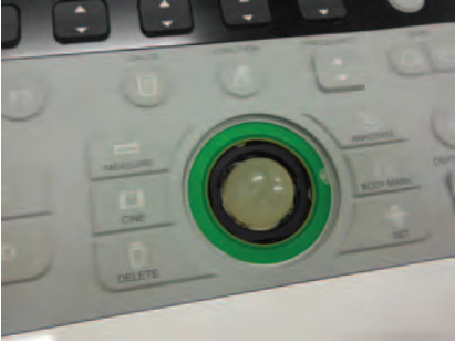
Figure 8-3: Trackball retainer removed
