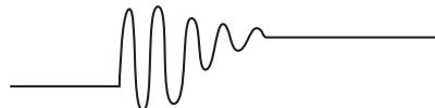
The signal oscillates between states after a mechanical switch or relay activates.
