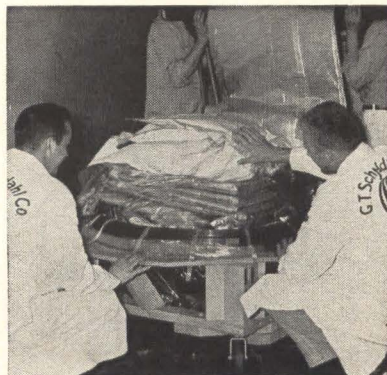
ECHO II passive communications satellite balloon is packed at G. T. Schjeldahl, Co., builder C
