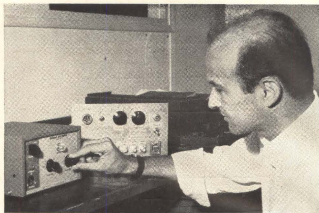
TESTING transistorized cardiac pacemaker
