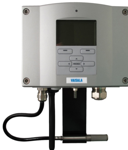
Figure 4 PTU301 Short Cable Probe
