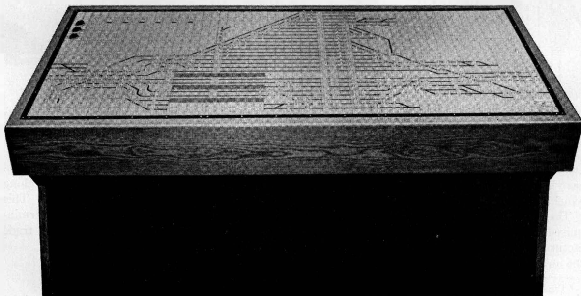
Figure 3—Typical track-diagram control desk consisting of 1512 mosaic elements.
