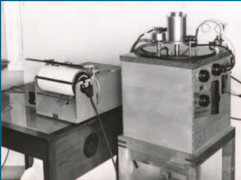
Calibration equipment for calibration of four radiosondes at a time, 1939.
