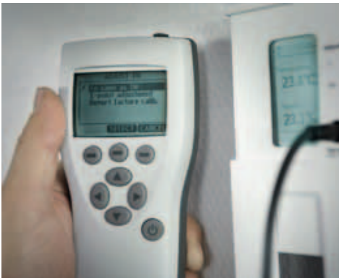
The transmitters can be easily calibrated without disturbing measurement performance. All it takes is a screwdriver and a reference instrument.
