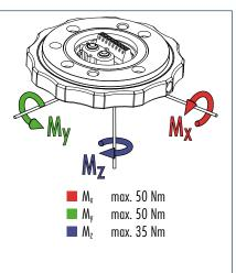
The dynamic moment load can be up to three times larger than the static moment load. Tests have shown that the system will only begin to fail in the event of 20-fold static moment.
