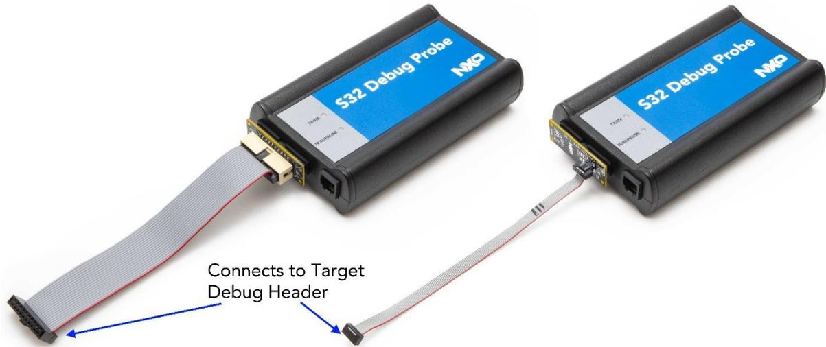
**Figure 7. S32 Debug Probe - connecting to target**
