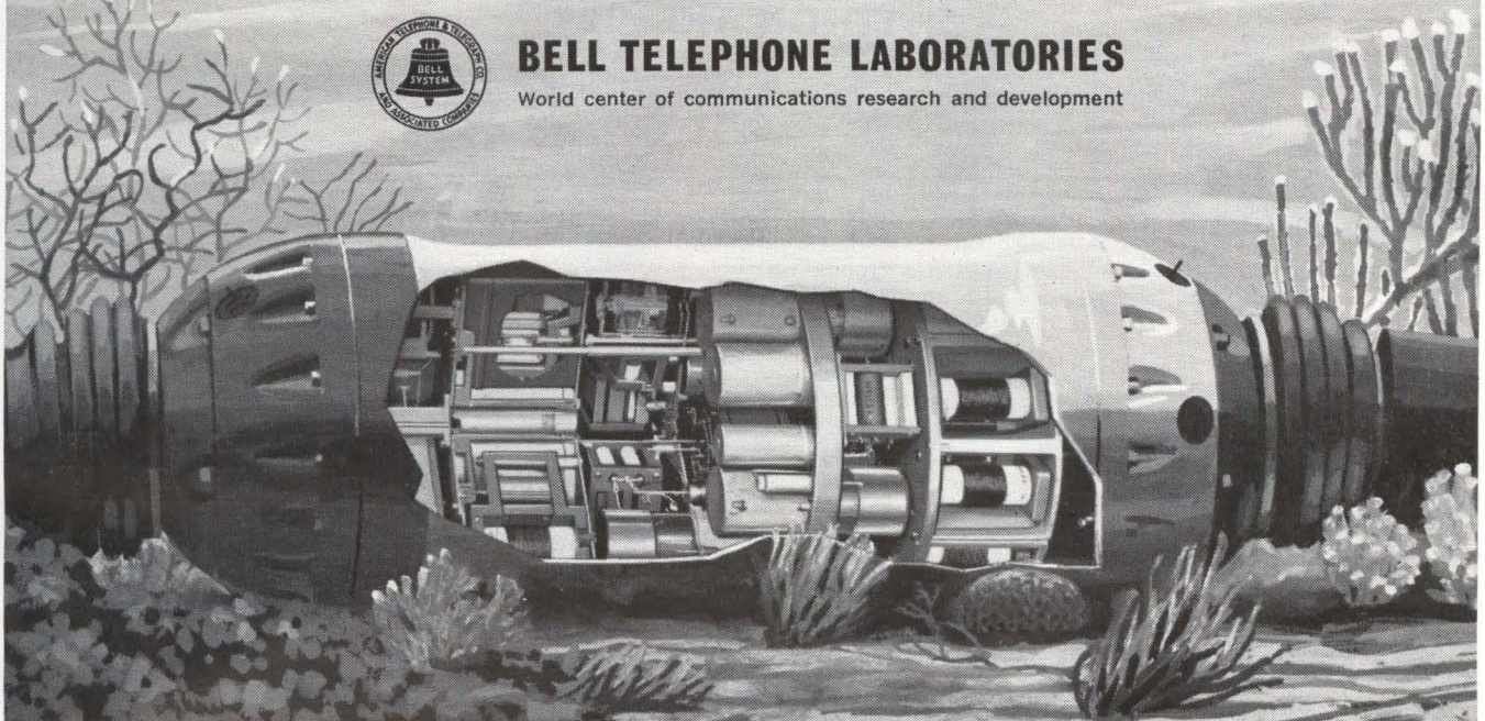
View of deep-sea amplifier with casing cut away. The casing is of noncorrosive beryllium copper, tested to withstand pressures up to 11,000 psi.
