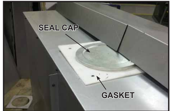
Figure 6.2 Seal Cap and Gasket Location
