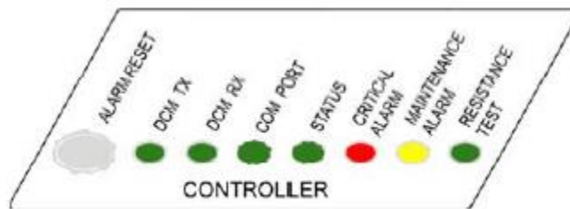
Figure 5. CM-XL8 Front Panel Indicators LEDs Explained
