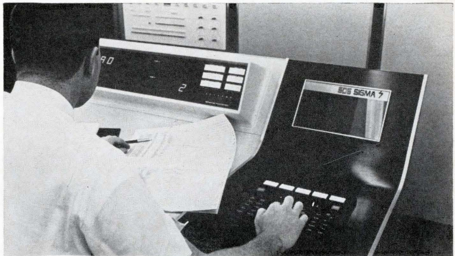
Programmer operates a keyboard to control time-sharing computer system of the Sigma 7.
