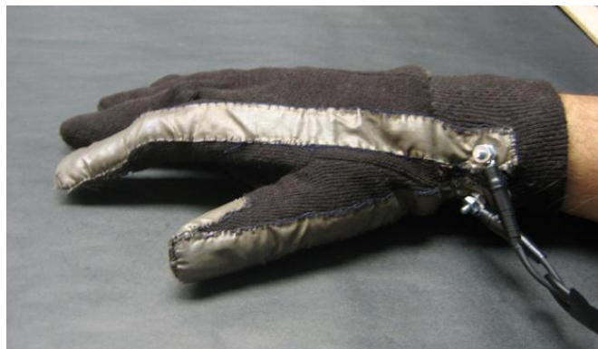
Figure 7.4: Instrumented gloves (right hand glove shown) designed by the author that produce an independent report for each of the user's two thumbs and two index fingers on the MERL DiamondTouch surface.
