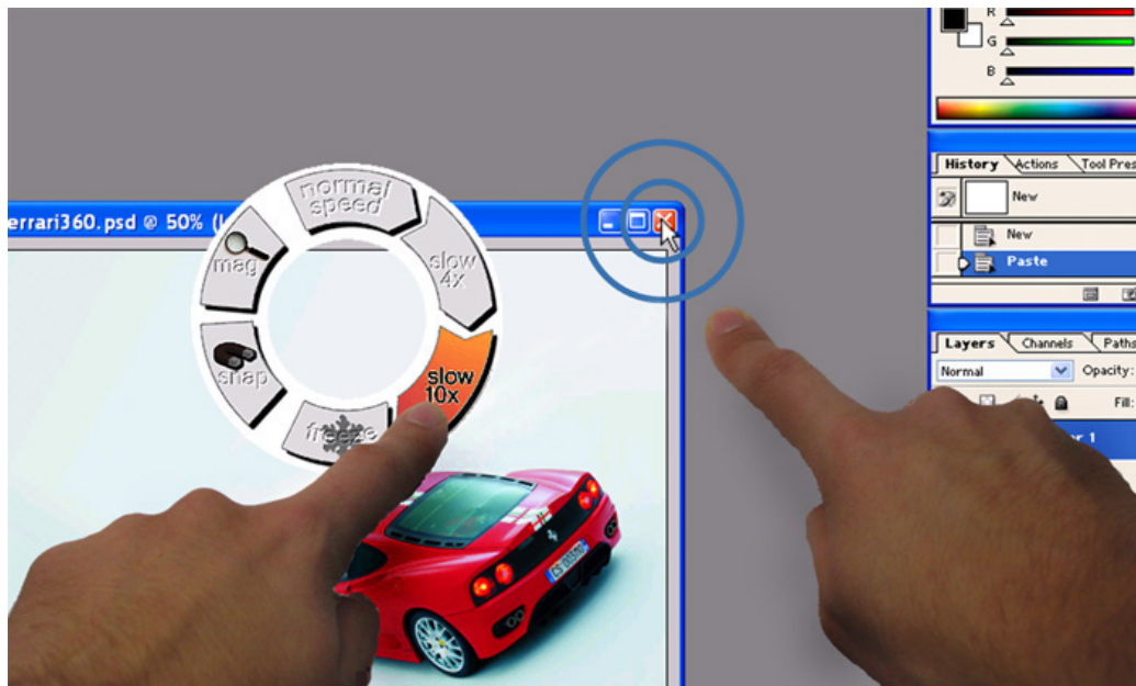
Figure 6.2: This image shows the use of the Dual Finger X-Menu in selecting “slow 10×” mode: the primary finger (right) controls the cursor position, while the secondary finger (left) adjusts the cursor speed.
