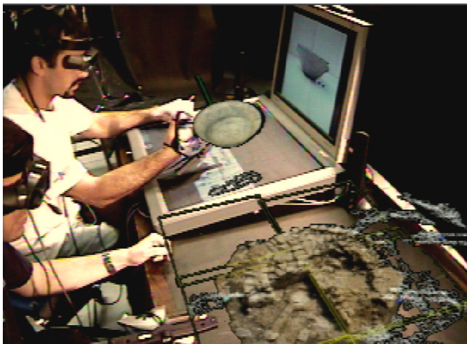
Figure 4.7: Two users simultaneously collaborate in VITA. While one user is inspecting the 3D virtual model of the ceramic vessel above the table, comparing it with the high-resolution image on the screen, the second user is looking at the 3D miniature terrain model next to the interactive tabletop.
