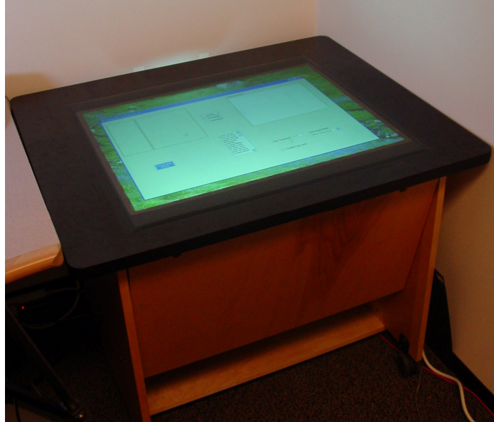
Figure 6.11: The multi-touch back-projected tabletop display prototype uses an infra-red illuminant and camera to detect contacts through a diffuse surface.
