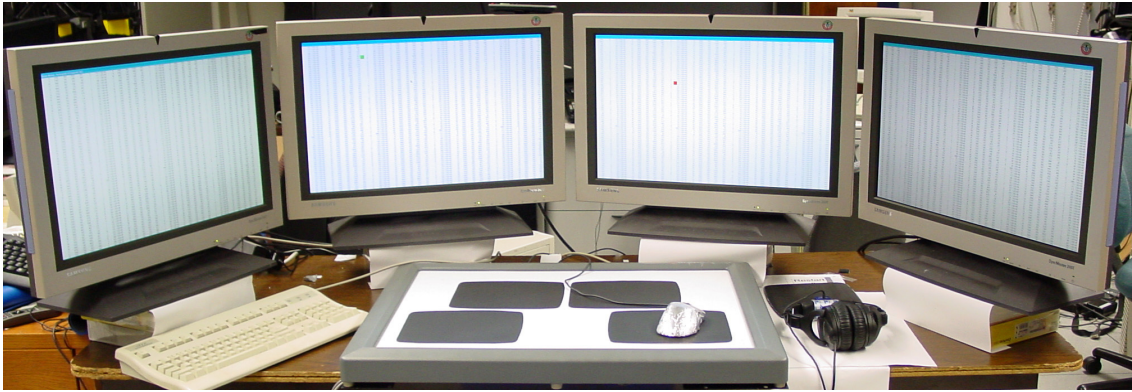
Figure 3.5: Experiment 1 setup: Homogeneous MDE test setup consisted of four monitors and four corresponding “mouse pads” used by mouse-location switch. The background is set to an inactive spreadsheet image to simulate a visually noisy working environment.
