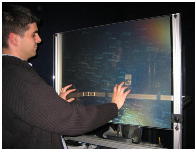
Figure 2.8: Using hand gestures to interact with map data on the TouchLight multi-touch prototype [Wilson 2004].
